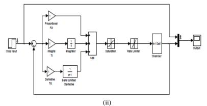
**Fig-13: block diagram for a continuous parallel PID controller**
