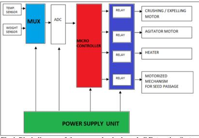
Fig-4: Block diagram of the proposed palm kernel oil Extraction System
