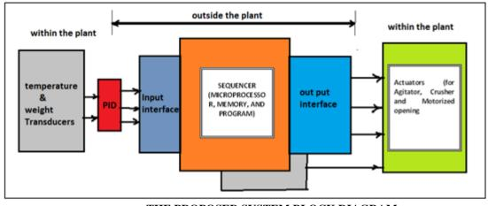
THE PROPOSED SYSTEM BLOCK DIAGRAM Fig-3: Block Diagram of the conceptualized palm kernel Extraction System
