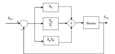
Fig-12: Block diagram of a continuous parallel PID controller
