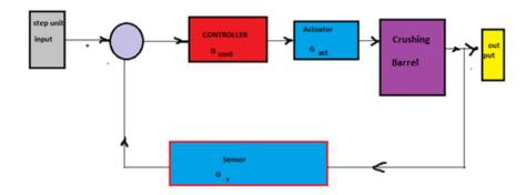
Fig-11 .Block Diagrame for Crushing Barrel Model
