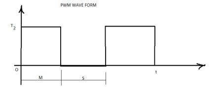
Fig-9: PWM Wave form for the blower to toasting drum.
