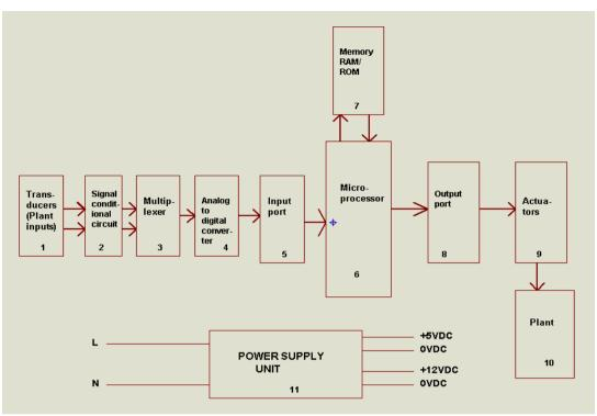
Fig-6: Detailed System Block Diagram
