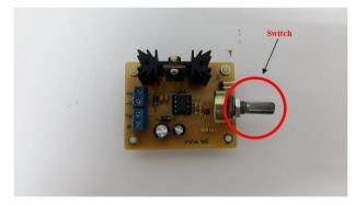
Fig-3: Pulse Width Modulation (PWM) device
