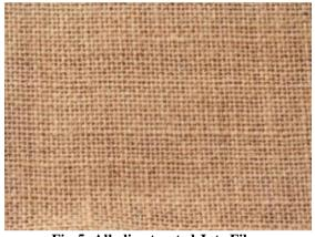
Fig-5: Alkaline treated Jute Fiber
