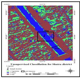
Fig-1: Unsupervised Classification appears pixel was a mixture water, vegetation and soil.
