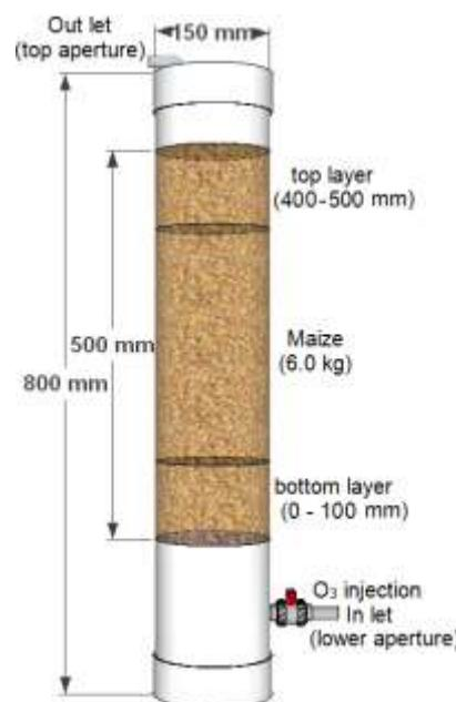
**Fig-1: Silo system for maize ozone treatment details and dimensions**
