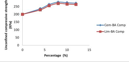
Figure 8: Plot of unconfined compressive strength versus soil composites
