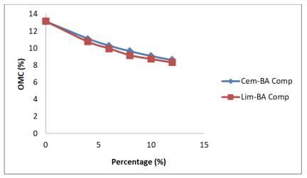
Figure 2: OMC versus stabilized soil composites
