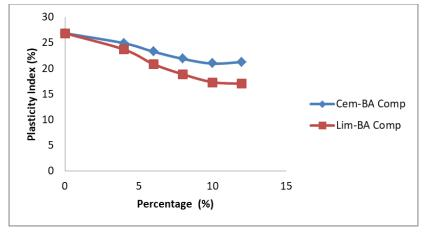
Figure 5: Plasticity index versus stabilized soil composites
