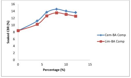
Figure 7: Plot of CBR for soaked sample versus stabilized soil composites
