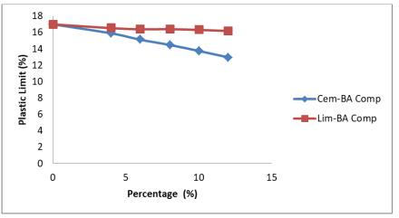
Figure 4: Plastic limit versus stabilized soil composites
