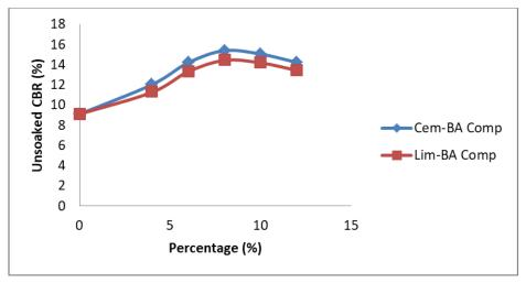
Figure 6: Plot of CBR for unsoaked sample versus stabilized soil composites
