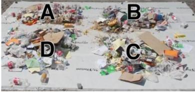
Figure 3: Quartering and Coning Techniques
