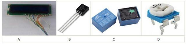
Figure 8: Liquid Crystal Display (A), Transistor (B), Relay (C), Variable Resistor (C) The Resistor R<sub>3</sub>: limits the current entering transistor Q1, MTN SIM, Light Emitting Diode, D4: indicates when the microcontroller is ready to function, Resistor, R4: limits the current entering into LED D4 and Variable Resistor (RV<sub>2</sub>): for contrast and controlling the display of the liquid crystal
