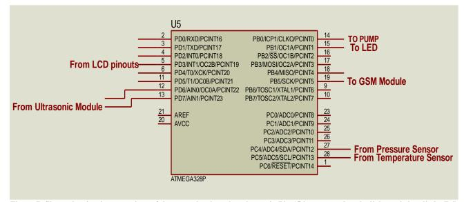
Figure 7: Shows the circuit connections of the control unit to the other unit. Pin 15 is connected to the light-emitting diode (D4) to indicate if the programming is working in the circuit. The resistor (R4) reduces the current that flows through the light-emitting diode (D4)
