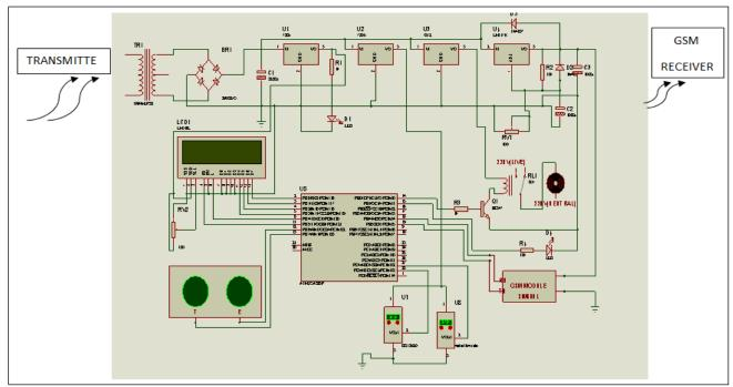
Figure 10: Circuit Diagram of water level monitoring.
