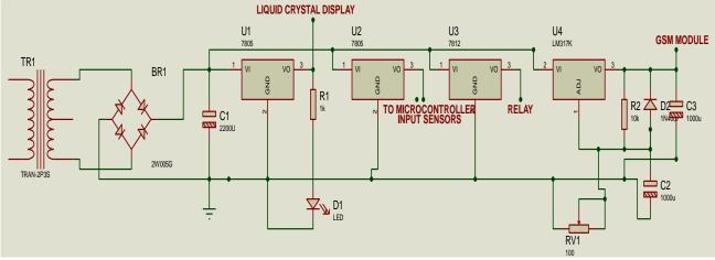
Figure 3: The complete circuit diagram of the power supply Unit
