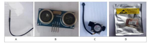
Figure 4: Water Proof Temperature Sensor (A), Ultrasonic Water Level Sensor (B), Flow Rate Sensor (C) and GSM Module (D) VBBKJ. The three sensors are used to convert the physical quantities they are sensing into electrical signal
