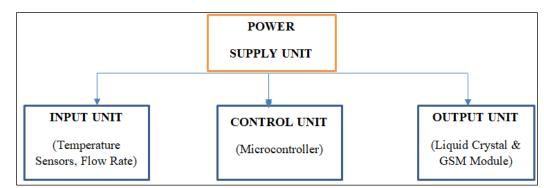
Figure 1: Block Diagram of Water Tank Level Monitoring System
