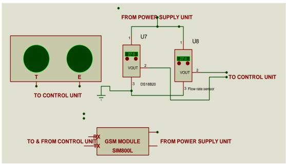
Figure 5: Circuit Diagram of Input Unit
