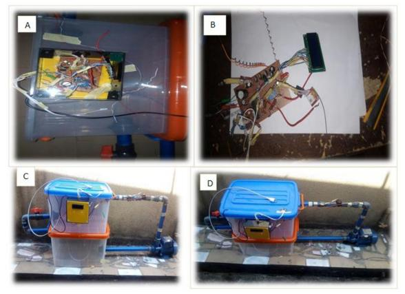
Figure 11: Microcontroller Circuit Connection (A) and Liquid Crystal Display Circuit Connection to Microcontroller (B). A bolt and nut were used to secure the transformer to the casing. The Vero-board is secured to the plastic shell using a bolt and nut. The system's tanks are made of two rubbers. Sensor and Microcontroller Mounting on the Tank (C), and Project Completion (D). After the packaging, the item was eventually tested and found to be functional
