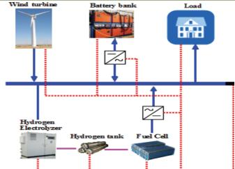
Figure 1.1: Schematic of Wind-Hydrogen-Fuel cell Hybrid System: Zachariah, et al., (2013)
