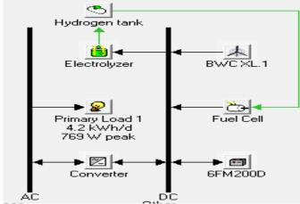
Figure 2.2: Schematic Diagram of Wind- Battery-Fuel cell hybrid System
