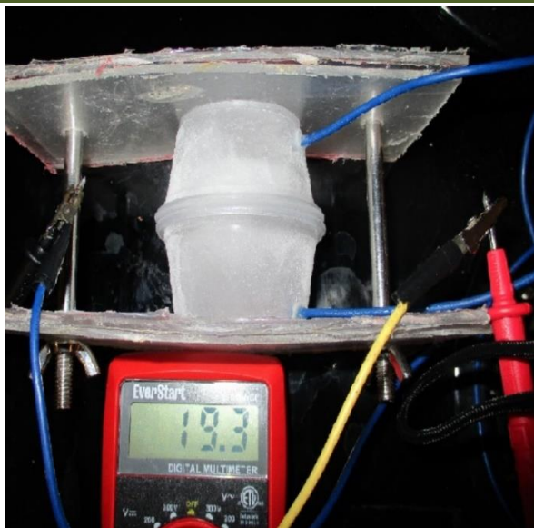
Figure 3: The installation is assembled. Two pieces of ice are tightly pressed together. Electrical wires are connected to the multimeter.
