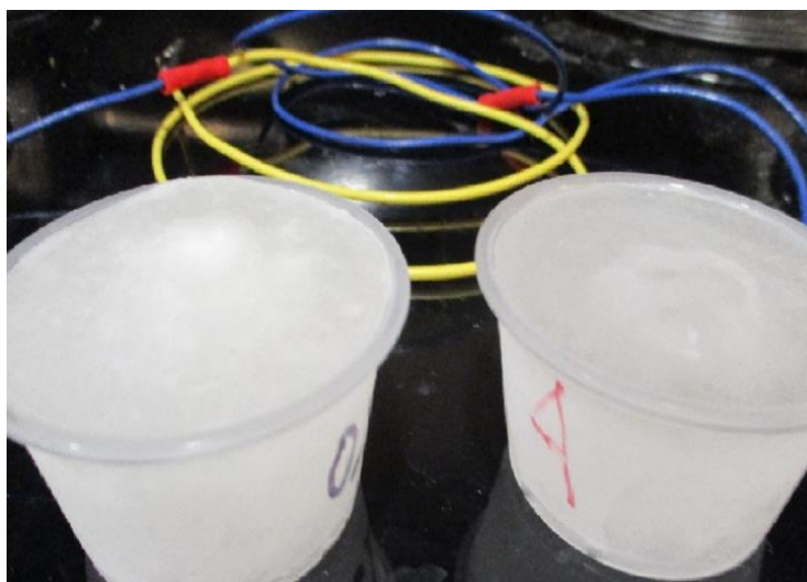
Figure 1: Plastic cups filled with aqueous acid and aqueous base solutions. The solutions are frozen in a freezer
