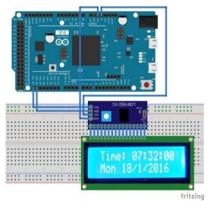
Fig-4: RTC circuit to Arduino Mega
