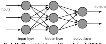
Fig-1: Multilayered feed forward Neural Network (MFNN)
