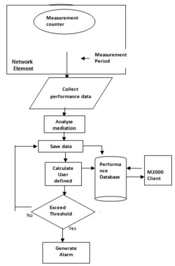
Fig-3: Process of performance measurement of the M2000system
