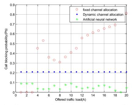
Fig-13: comparison of fixed channel allocation, Dynamic channel allocation and artificial neural network
