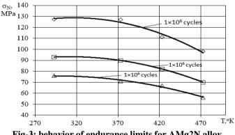
Fig-3: behavior of endurance limits for AMg2N alloy
