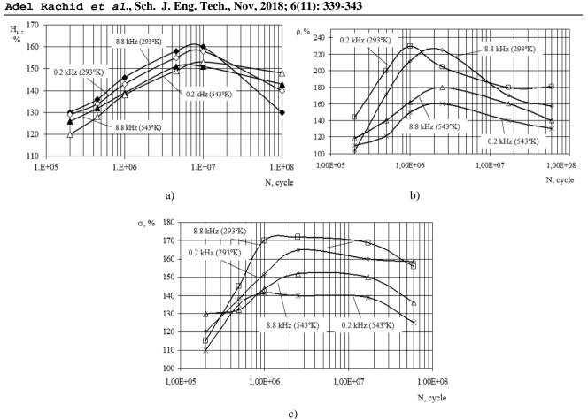
Fig-4A: Kinetics micro-hardness for Copper M1; B) Kinetics of dislocation density Copper M1; C) Kinetics micro strain for Copper M1
