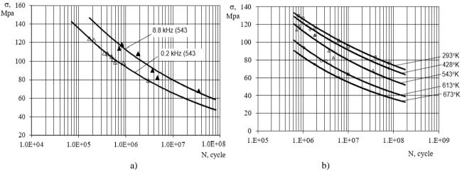
Fig-1: Fatigue curves of copper M1at: a) different frequencies; b) different temperatures and 0.2 KHz.
