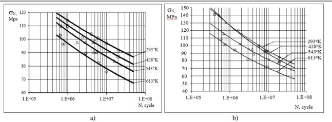
Fig-2: Fatigue curves with test frequency 8.8 kHz for: a) alloy D16; b) AMg2N alloy
