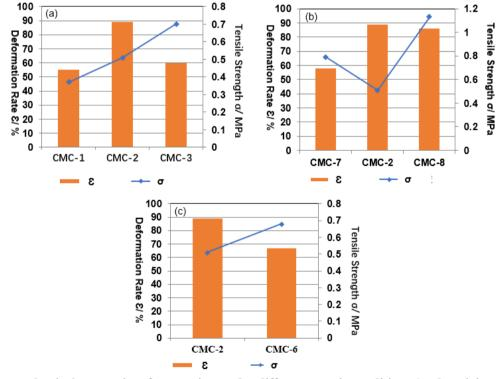
Fig-1: The mechanical properties of composites under different matrix conditions (a: the mixing time; b: the content of SiO<sub>2</sub>; c: frozen or not)
