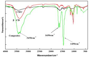
Fig-4: The FTIR spectrogram of CMC, β-CD, and β-CD/CMC membrane composites
