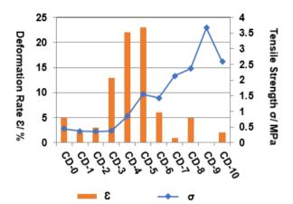
Fig-2: The mechanical properties of composites under different β-CD content
