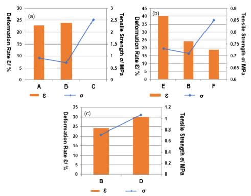
Fig-3: The mechanical properties of composites with 0.5g β-CD added under different matrix conditions (a: the mixing time; b: the content of SiO<sub>2</sub>; c: frozen or not)
