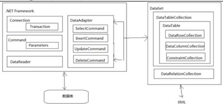
Fig-1: Model structure of ADO.NET
