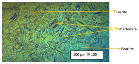
Fig-13b: Sample of D= 25mm, H= 40mm @ surface temperature 500<sup>o</sup>C
