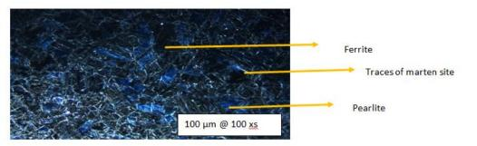
Fig-12a: Sample of D= 20mm, H= 70mm @ surface temperature 469<sup>o</sup>C
