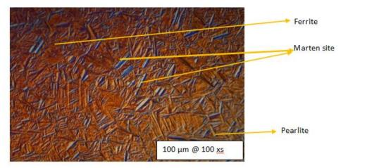
Fig-12d: Sample of D= 45mm, H= 70mm @ surface temperature 438<sup>o</sup>C
