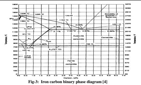
A fully pearlite microstructure is formed at the eutectoid composition of 0.78% C. as can be seen in figs.4 and 5, pearlite forms as colonies where the
