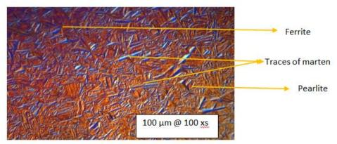
Fig-12c: Sample of D= 32mm, H= 70mm @ surface temperature 440<sup>o</sup>C
