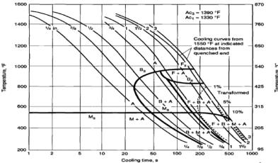
Fig-6: The CCT Diagram for type 4340 Steel Austenitized at 845°C [3]
