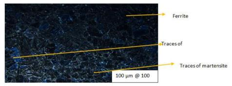
Fig-13a: Sample of D= 20mm and H= 40mm @ surface temperature 500<sup>o</sup>C
