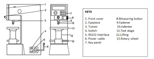
Fig-11: Rockwell Hardne Test Machine
