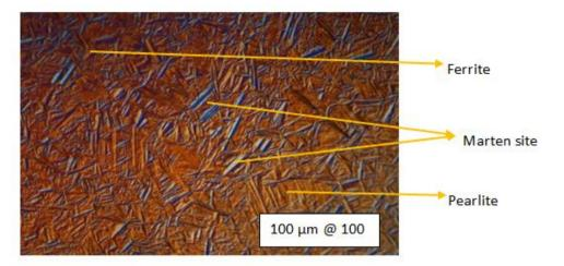
Fig-13c: Sample of D= 32mm, H= 40mm @ surface temperature 470<sup>o</sup>C
