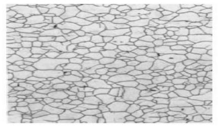
Fig-2: Microstructure of fully ferrite of low carbon steel [3]
