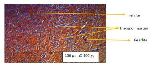
Fig-13d: Sample of D= 45mm, H= 40mm @ surface temperature 458<sup>o</sup>C
