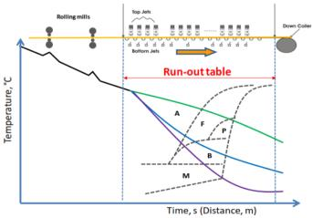
Fig-1: Schematic of hot rolling mill of steel plates and strips. The schematic plot shows temperature variation versus time and its effect on the phase transformation of austenite decomposition. A: austenite, F: ferrite, P:
