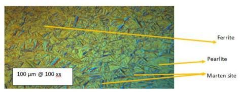
Fig-12b: Sample of D= 25mm, H= 70mm @ surface temperature 463<sup>o</sup>C
