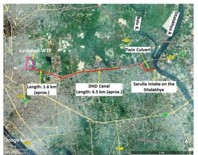
Fig-1: Raw water source and its transmission network from Sitalakhya river through DND canal to plant
