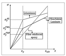
Fig-3: Schematic illustration of Stress-Strain curves
