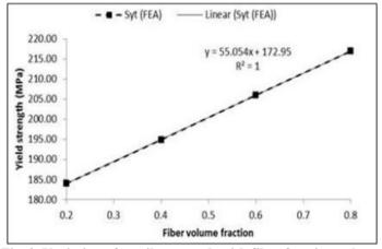
Fig-4: Variation of tensile strength with fiber fraction volume
