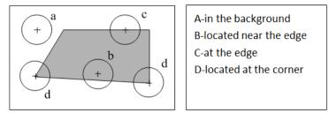
Fig-1: The schematic diagram of SUSAN corner detection
