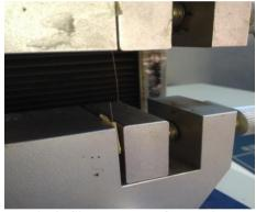
Fig-3: Single strand after testing
