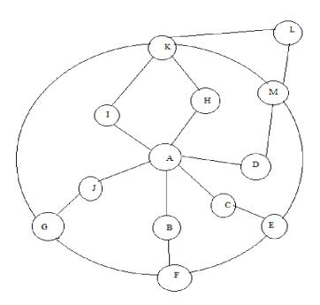
Fig. 2: Routing Zone of Node A with Radius ρ=2 hop
