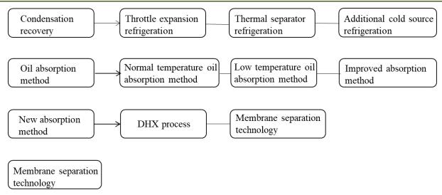
Fig-2: Different light hydrocarbon recovery technology classification
