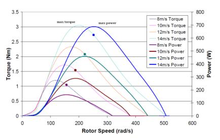
Fig-17: Coleration of between Torque, Rotor speed and Output Power
