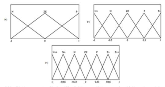
Fig-11. a-) The first input membership functions, b-) the second input membership functions c-) the output membership functions
