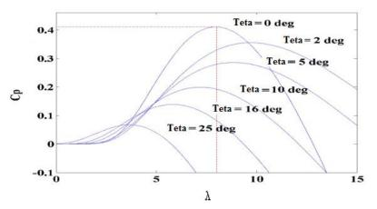
Fig-16: Coleration of between Cp (performance coefficent) and  $\lambda$  (Tip speed ratio) in different values of pitch angle ( $\theta$ )
