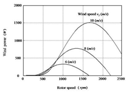
Fig-15: Corelation of wind speed, rotor speed and wind power values
