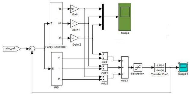
Fig-13: Fuzzy-PID controller simulink model
