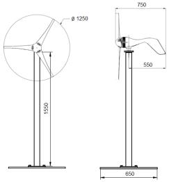
Fig-1: Turbine views and dimensions
