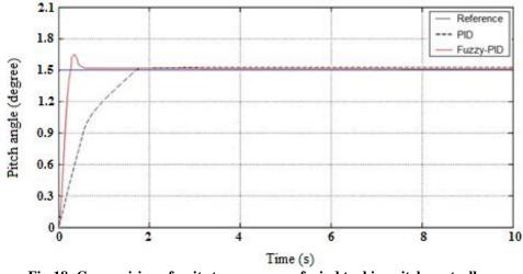
Fig-18: Comparision of unit step response of wind turbine pitch controllers
