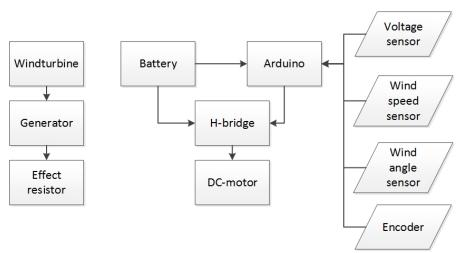
Fig-14: Block diagram of the system and ardunio
