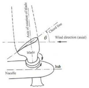
Fig-5: Pitch angle of blade in wind turbine
