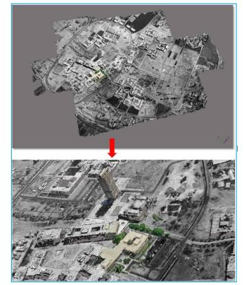
Fig-9: The Dense point cloud of the virtual city model of COE in UOB campus
