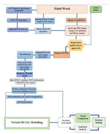
Fig-3: Workflow diagram of the research methodology
