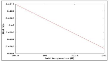
Fig-8: Effect of Compressor Inlet Temperature on Work Ratio of the Gas Turbine Generator
