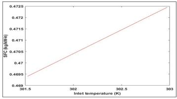
Fig-7: Effect of Compressor Inlet Temperature on Specific Fuel Composition of the Gas Turbine Generator
