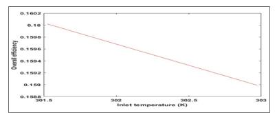
Fig-3: Effect of Compressor Inlet Temperature on the Overall Efficiency of the Gas Turbine Generator
