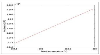
Fig-5: Effect of Compressor Inlet Temperature on the Heat Rate of the Gas Turbine Generator
