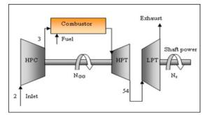
Fig-1: Two shafted Gas Turbine with Sensor Placement
