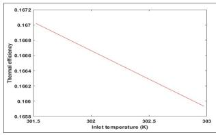
Fig-4: Effect of Compressor Inlet Temperature on the Thermal Efficiency of the Gas Turbine Generator
