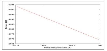
Fig-6: Effect of Compressor Inlet Temperature on the Thermal Power of the Gas Turbine Generator
