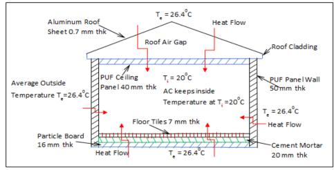
Fig-3: A sketch showing the construction details and heat flow
