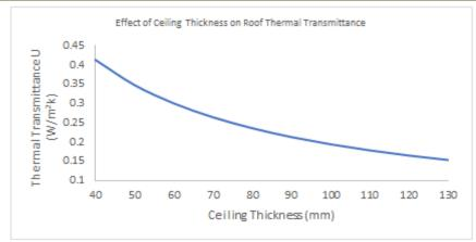
Fig-7: Effect of Ceiling Layer Thickness on Roof Thermal Transmittance
