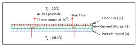
Fig-6: A sketch showing the floor thermal layers
