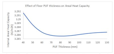
Fig-17: Effect of Floor PUF Layer Thickness on Floor Areal Heat Capacity
