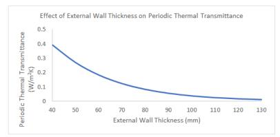
Fig-13: Effect of Wall Layer Thickness on Wall Periodic Thermal Transmittance
