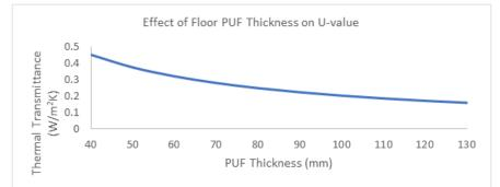
Fig-16: Effect of Floor PUF Layer Thickness on Floor Thermal Transmittance
