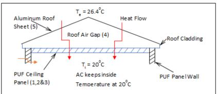
Fig-5: A sketch showing the roof and ceiling thermal layers
