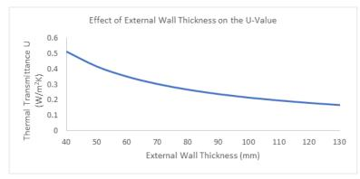
Fig-11: Effect of Wall Layer Thickness on Wall Thermal Transmittance
