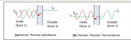
Fig-1: Illustration of Thermal Admittance and Periodic thermal Transmittance
