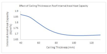
Fig-8: Effect of Ceiling Layer Thickness on Roof Areal Heat Capacity
