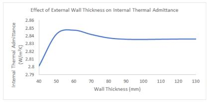
Fig-14: Effect of Wall Layer Thickness on Wall Thermal Admittance
