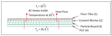
Fig-15: A Sketch of modified Floor Construction and thermal layers
