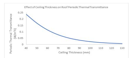
Fig-9: Effect of Ceiling Layer Thickness on Roof Periodic Thermal Transmittance
