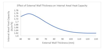
Fig-12: Effect of Wall Layer Thickness on Wall Areal Heat Capacity
