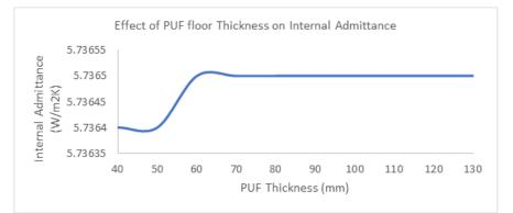
Fig-18: Effect of Floor PUF Layer Thickness on Floor Thermal Admittance
