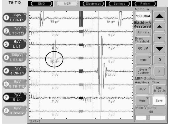
Fig-2: Channel 4 shows an amplitude of 100 µV, which is an 80% decrease in value (black empty circle) compared to the normal MEPs response before compression and distraction.
