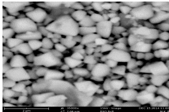
Fig-2: SEM micrograph of sample oxidised at 1050°C for 3 min. and annealed at 500°C for 90 min after etching
