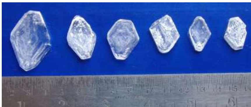
Fig-1: Photograph showing the pure and Magnesium Chloride added DSHP crystals grown [From left are: 0.0 (pure DSHP), 0.2, 0.4, 0.6, 0.8 and 1.0 mole% MgCl 2 added]
