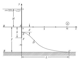
Fig 1b: The current picture calculated at  $\varepsilon = 0.6$ , T = 7, S = 3, H = 7, H<sub>0</sub> = 3  $\mu$  x<sub>C</sub> = 100
