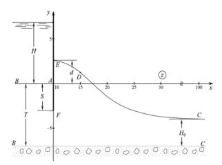
Fig 1a: The current picture calculated at  $\epsilon$  = 0.6,  $h_c$  = 0.5, T = 7, S = 3, H = 5
