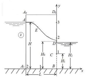
Fig 2: The current picture in a rectangular jumper calculated at  $\varepsilon = 0.5$ , H = 3, L = 2,  $H_1 = 1$ ,  $H_2 = 1.4$
