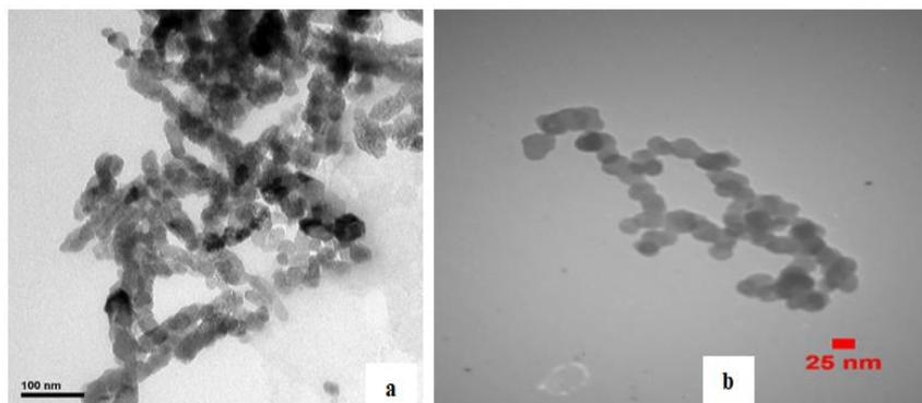
**Figure 2:** a) Transmission electron microscopy of silver nanoparticles synthesized from the extract of yogurt enriched with *Lactobacillus* flora with magnification of 25 b) microscopic image of field emission scanning electron of silver nanoparticles synthesized from the extract of yogurt enriched with *Lactobacillus* flora with magnification with magnification of 100
