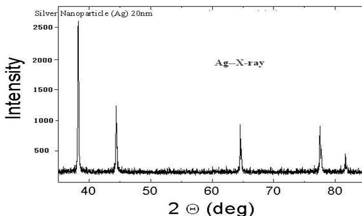
**Graph 1:** XRD test of nanoparticles
